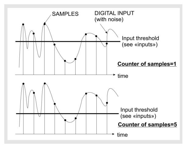
If counter of samples is greater than (or equal to) reg.40046 (Filter Sup), input signal is detected as "1".
