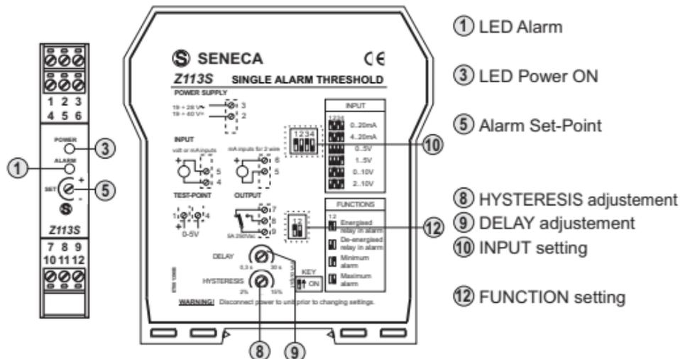
Programming for INPUT SETTING and for FUNCTION SETTING must be done when unit is not powered.
