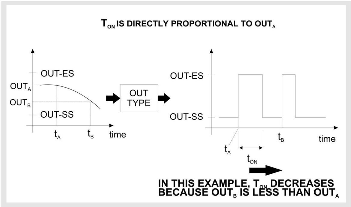
It is possible to limit upper time of high-state ON/OFF output (reg.40029) and to limit lower time of low-state ON/OFF output (reg.40030). The cycle time is reg.40028 (constant frequency of ON/OFF output=1/cycle time).
