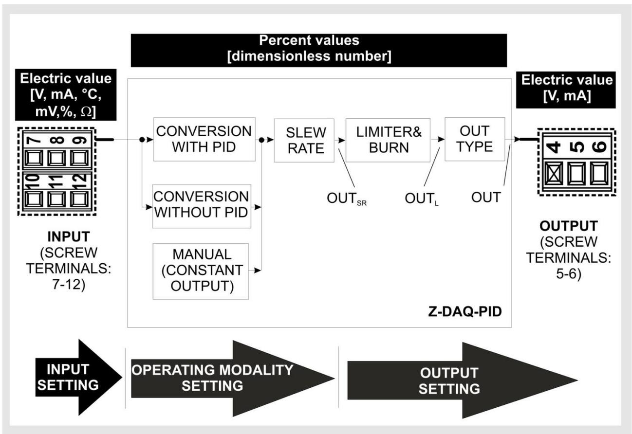
In particular, there are three operating modes, each of them allows to supply a ON/OFF output or an analog output:
