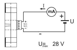
t is possible to connect directly on the  $4 \div 20$  mA loop in T201DC100 output a maximum voltage of 28 V.
