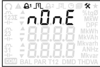
At first User setup access, the digital output is disabled (NONE) and no parameter is associated. To enable the digital output, press **◀** button, the NONE item will start to blink. With **▲** or **▼** button select the mode (**AL H**, **ALL**, **PULS**). Confirm with **◀** button.
