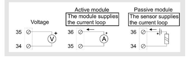
Shielded cables are recommended to connect the outputs.
