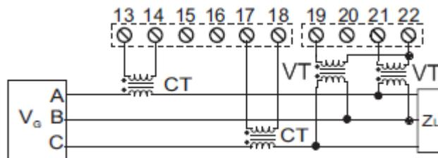
**2.8. 4 wire with neutral insertion with CTs (4 wires insertion)**
