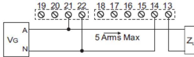
**2.3. Single phase insertion with CT (1-phase insertion)**
