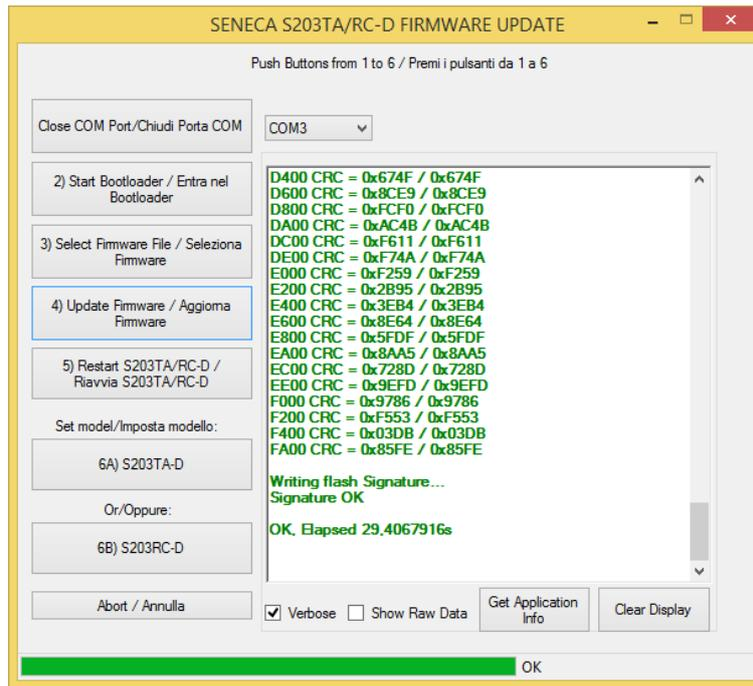
Press the 5) button to restart the S203TA/RC-D, now the board is out of the bootloader mode.
