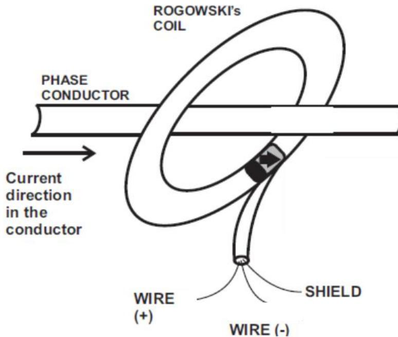
Rogowski's coil have been designed for accurate nonintrusive measurement of AC, pulsed DC or complex waveforms.
