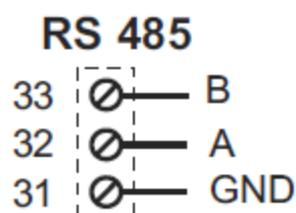
There is no insulation between RS485 and the analog output
