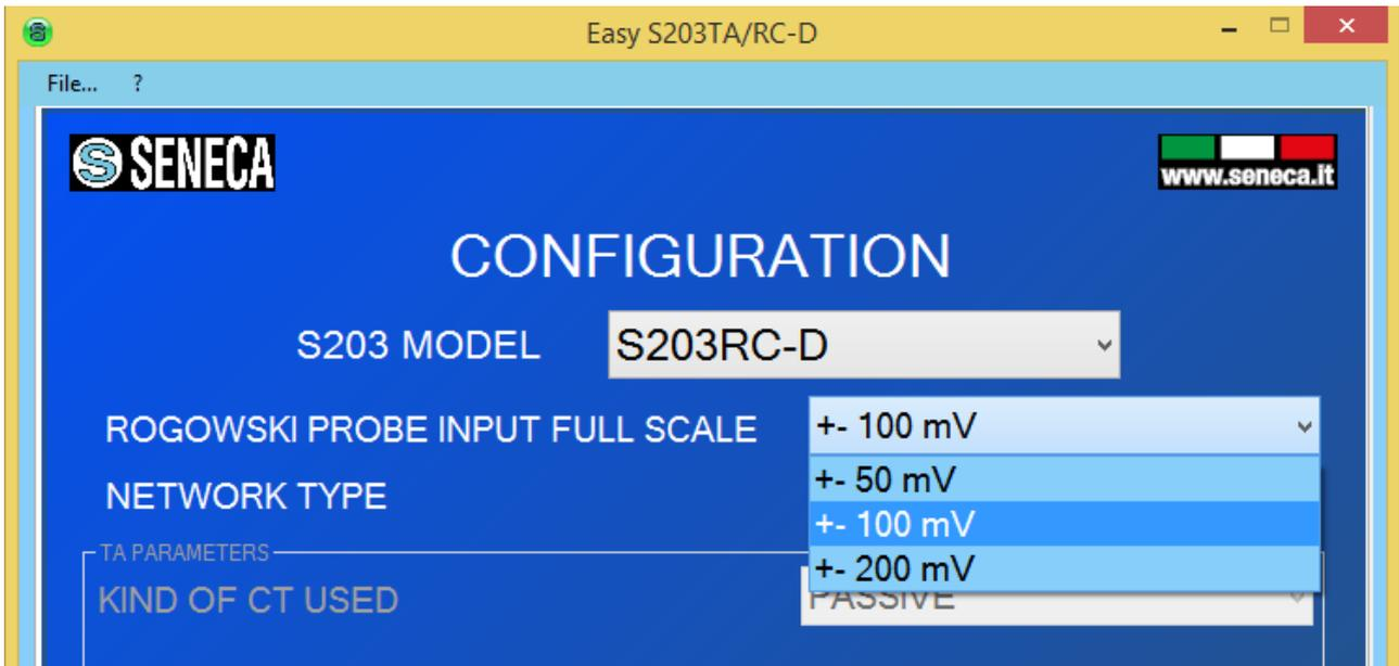
Set the right full scale on S203RC-D for various Rogowski coil type and/or the user tarature multiplication factor for current phase A,B and C (From Easy Setup software or by menu -> user tarature->current phase A,B,C).
