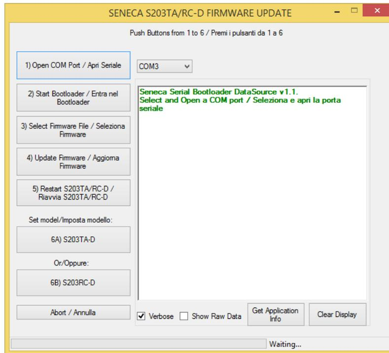
Press the 1) button for connect to the right S203TA/RC-D serial port
