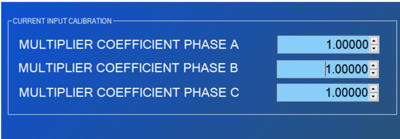
For use with a different Rogoski Coil Model you must calculate the right coefficient using this formula (Note that the “Rogowski Probe Input Full Scale [mV]” can only be 50,100 or 200 mV):
