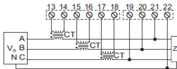
**2.9. 3-phase without neutral insertion with CTs (4 wires insertion)**
