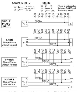
Note: You can't connect the secondary of any CTs to the Earth. Terminals 14, 16 18 and 22 are internally connected.
