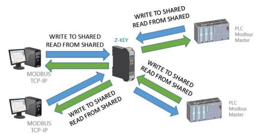
The shared memory of the gateway can be freely read and written by the Ethernet and/or by the serial ports.
