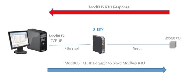
The Modbus TCP Client requests the reading/writing of a Modbus register via Ethernet, the gateway converts the request towards the serial slaves in Modbus RTU/ASCII and the Modbus RTU/ASCII response of the interrogated slave is subsequently converted towards the Modbus TCP Client.
