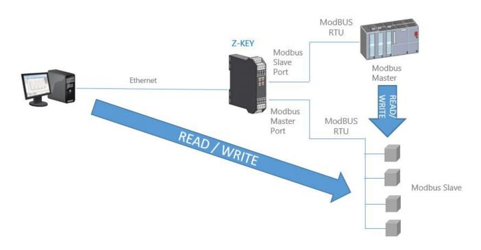
This function is possible because the Seneca Gateway uses an internal memory shared between the serial ports and the Ethernet port, where the data acquired from the serial Modbus Slave network are saved. The Modbus Master PLC and the PC write/read the registers of the shared memory of the gateway which in real time keeps it updated by communicating with the Modbus Slaves.
