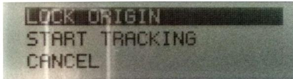
You can now select an option from the menu using the SCR key and confirming with the left PWR key.
