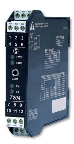
VOLTAGE INPUT: 0..1.200 Vdc; 0..850 Vac
