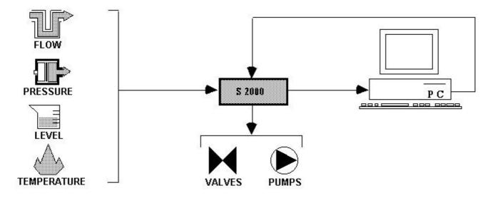
The signals from transducers go to the analogue inputs of the S2000, which in its turn can use them or otherwise in required logic-mathematical operations and then retransmit the corresponding values via serial line to the PC for display. The PC can also transmit to the S2000 module via serial line the required information for control of devices such as valves or pumps, connected to the analogue outputs of the module itself.
