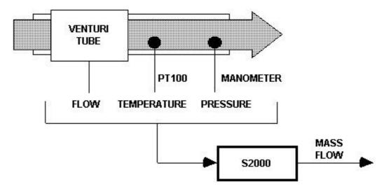
The S 2000 module can provide an output analogue signal proportional to the above mass, combining the gas flow rate, measured by means of a Venturi pipe or a calibrated flange or a Vortex etc., with the temperature and pressure of the gas.
