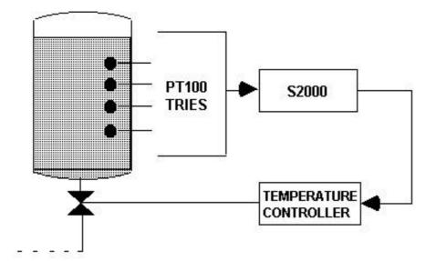
The S2000 module can assess the mean of the values corresponding to the analogue signals from the probes and control a temperature regulator on the basis of this mean.
