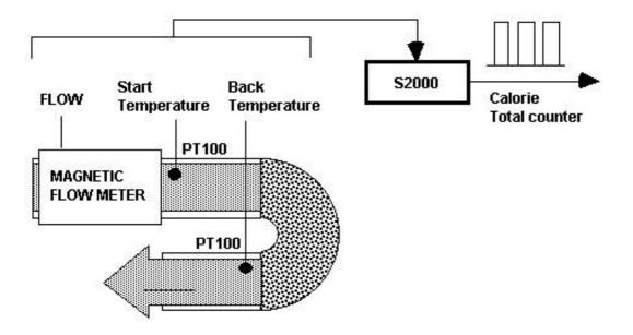
As a calory counter the S2000 is able to totalise the thermal energy developed in a pipe used for heating, for example, calculating the difference between the two temperatures, high and low, provided by two PT100 probes and multiplying it by the flow rate of the pipe measured by means of a magnetic meter.
