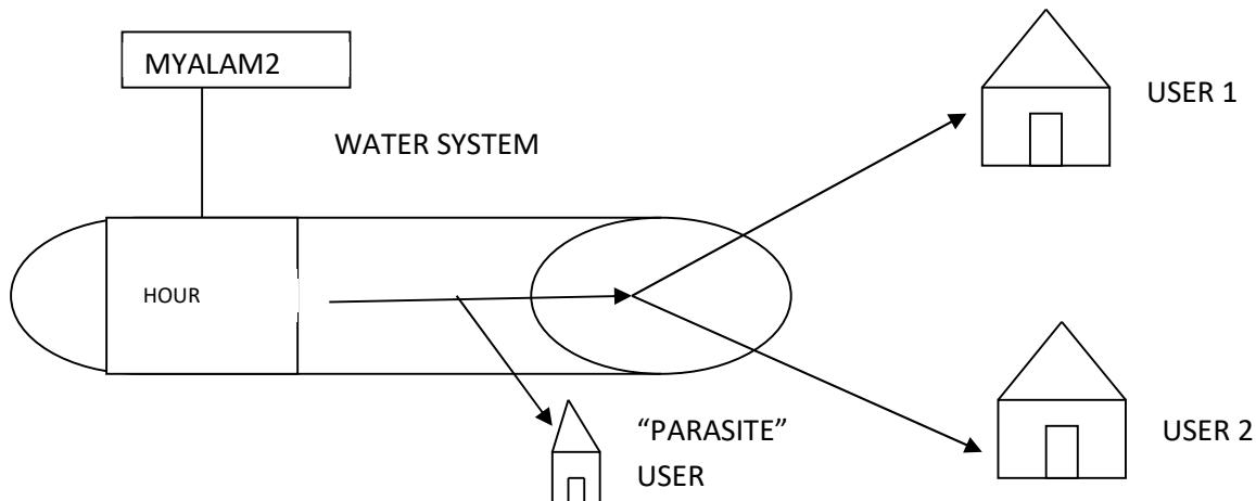
If this is not the case it means that there is a "parasite" utility in addition to the 2 utilities that continuously subtracts liquid (especially at night it is improbable that the utilities use water on all the 10 minute intervals).
