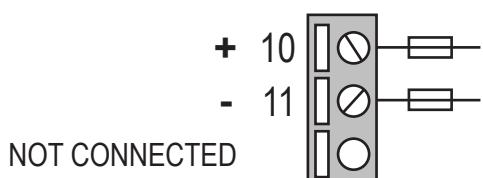
The power supply must be connected to terminals 10 and 11. The supply voltage must be: 10 to 30Vdc, It is advisable to insert a 1 A delayed fuse
