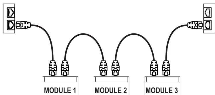
There must be no loops in the Ethernet cabling, otherwise the communication will not work. The modules and switches must be connected eliminating any loops. The following examples show the incorrect connections.
