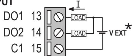
The device has two digital outputs. Range:  $I_{max} = 50 \text{ mA}$   $V_{max} = 28\text{V}$ . See user manual for functionality.
