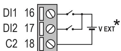
The device is equipped with two digital inputs that can be activated with voltage from 12 to 24 V. See user manual for functionality.
