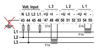
The same circuit diagram can be applied for connections of Rogowski sensors and CTs with mV outputs.
