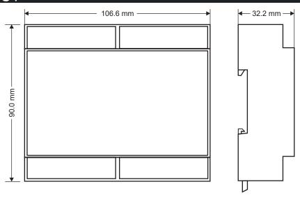
Weight: 170 g; Enclosure: UL94-V0 self-extinguishing PC/ABS material, black.
