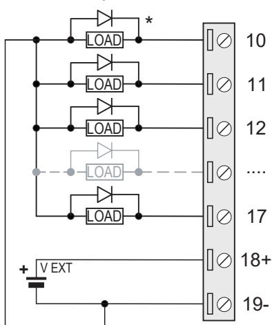
The digital outputs must be powered externally to function properly (V EXT).
