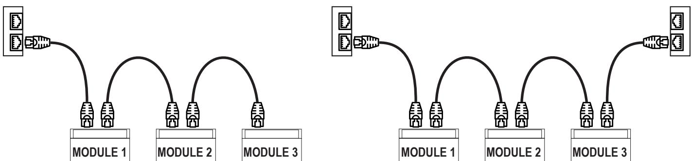
There must be no loops in the Ethernet cabling, otherwise the communication will not work. The modules and switches must be connected eliminating any loops. The following examples show the incorrect connections.
