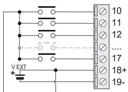
The digital inputs must be powered externally to function properly (V EXT).
