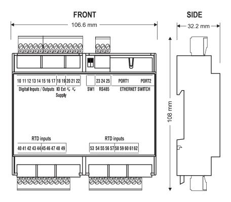
Weight: 170 g; Enclosure: UL94-V0 self-extinguishing PC/ABS material, black.
