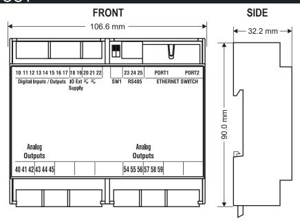
Weight: 170 g; Enclosure: UL94-V0 self-extinguishing PC/ABS material, black.
