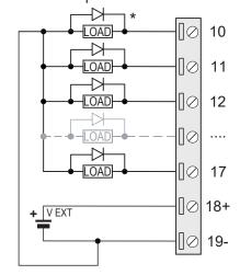
The digital outputs must be powered externally to function properly (V EXT).
