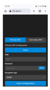
7) To search for the router's wifi network to which the control unit will connect, press the "SCAN" button to start the network scan process:
