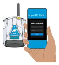
6) You can now manually enter the router's Wi-Fi network to connect to the internet, or search for it automatically. It is possible to insert up to two different Wifi routers (primary and secondary), in case of failure of connection to the primary the control unit will connect to the secondary. If you want to use a single wifi router leave the secondary empty.
