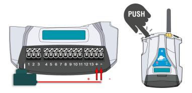
3) Start-up: At this point the control unit turns on and the writing "WIFI ACCESS POINT" will appear on the display, the "NET" LED flashes continuously and the control unit is therefore ready to accept the WIFI connection of a smartphone for the first configuration.
