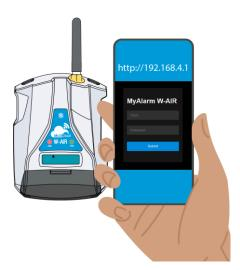
5) It is now possible to manually enter the router's wifi network or search for it automatically. It is possible to insert up to two different Wifi routers (primary and secondary), in case of failure of connection to the primary the control unit will connect to the secondary. If you want to use a single wifi router leave the secondary empty.
