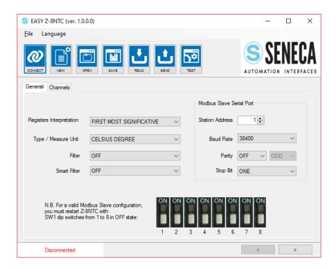
**Registers Interpretation:** Select from Most Significant First (Big Endian) or Less Significant First (Little Endian) for the Floating Point Measure Modbus Registers. This parameter affects only the Floating Point measurement registers.
