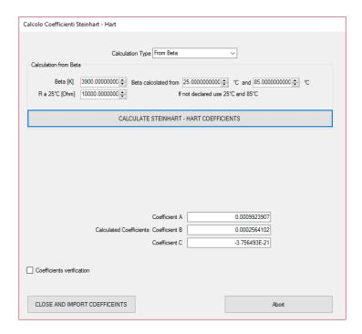
The NTC sensor datasheets usually do not provide directly the Steinhart-Hart coefficients. The most used is the Beta value, other times, they provide a temperature / resistance table directly.
