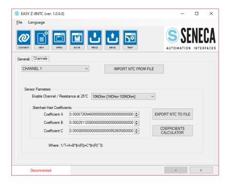
In the channel tab you can select the NTC parameters for each channel.
