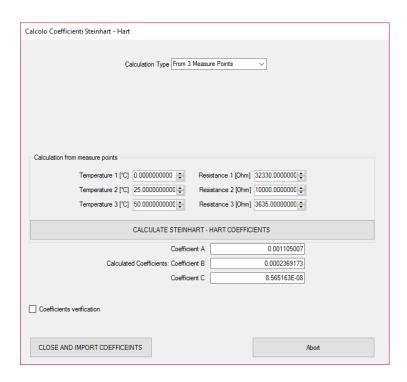
Possibly select 3 points equally spaced in your measure range, for better precision insert also the value at 25°C.
