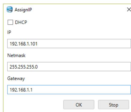
Confirm with OK. Now the device can be reached via Ethernet from your PC.
