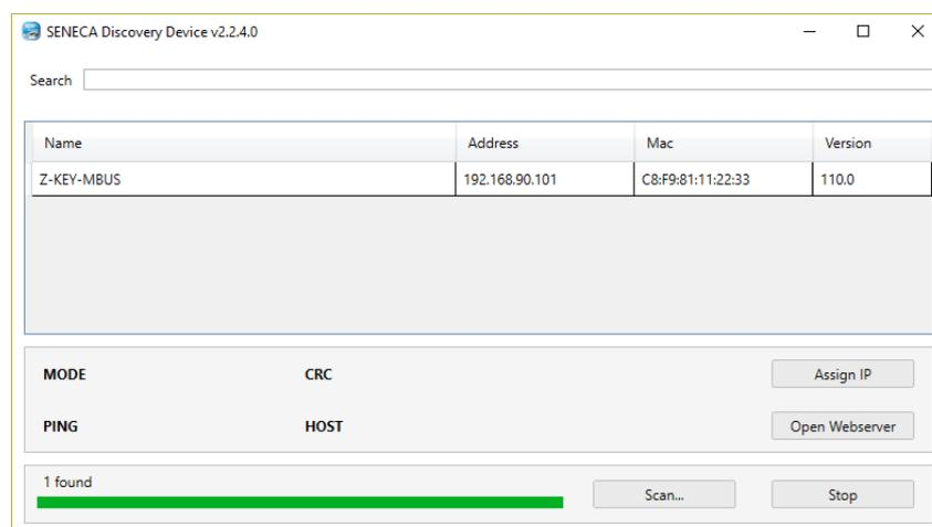
The software works at Ethernet Layer 2 level and it is therefore not necessary to have an Ethernet configuration compatible with the device you are looking for.
