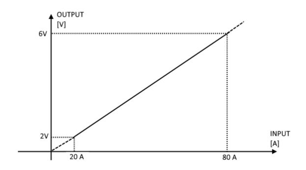
Note that with an input of 0A, the output is 0V and with a value greater than 80A, the output is greater than 6V (6V and 2V are not a limit).
