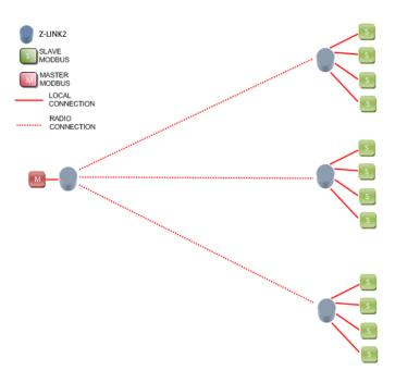
It is also possible to connect Modbus Slaves on the local Modbus master bus:
