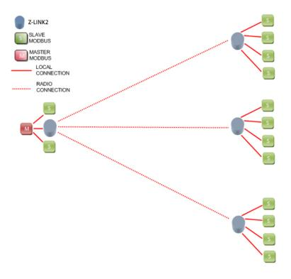
If a Z-LINK2-LO is not easily accessible, it is possible to configure one as a "repeater", note that Modbus RTU Slave devices can also be connected to the repeater:
