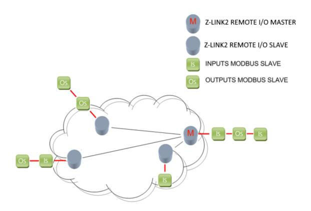
The inputs are replicated on the outputs. If the inputs are digital it is possible to negate them, if they are analogue it is possible to scale their values. A fault condition can be used for safety requirements.
