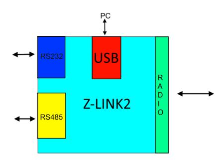
The Z-LINK2-LO USB port can only be used for programming Z-LINK2-LO from a Windows™ PC with the Easy Setup software.
