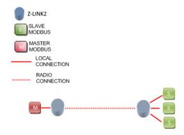
Furthermore, it is possible to connect 1 Modbus master without local Modbus slaves (point-to-multipoint):
