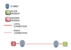
More complex, it is possible to connect 1 Modbus master with multiple Modbus slaves:
