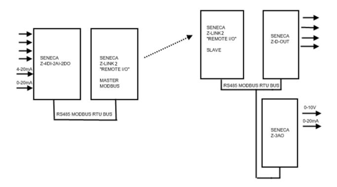
Digital inputs can be negated before retransmission while analogue measurements can be scaled before retransmission.
