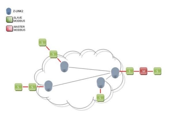
In this mode the Modbus fieldbus is transparently connected "over the air".
