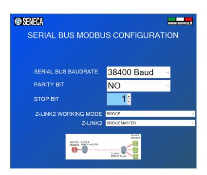
The Z-LINK2-LO connected to the Master is called "Bridge Master", while the other Z-LINK2-LOs (connected to the slaves) are called "Bridge Slaves".
