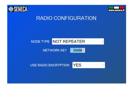
It is possible to choose if the device is of the repeater type, the network key and if the radio packets are encrypted.
