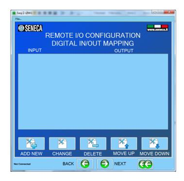
Press "Add new" and select from the internal Seneca database the digital input that must be retransmitted to the output:
