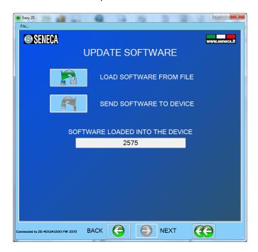
By pressing the "Load software from file" button, the software will open the firmware directory.
