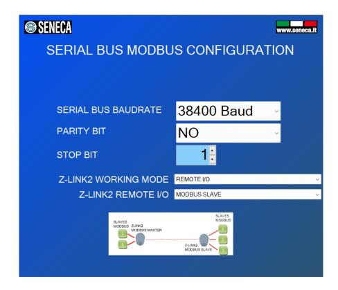
The Z-LINK2-LO acting as Modbus Slave is called "Remote I/O Modbus Slave".
