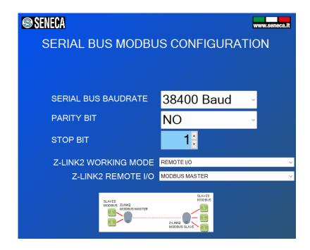
The Z-LINK2-LO acting as Modbus Master is called "Remote I/O Modbus Master".
