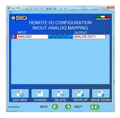
6) Once the configuration has been sent to the Z-LINK2-LO, turn off the device and set the dip switches:
