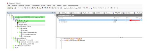
while to write the outputs you just set the byte value in the "prepared value" column, for example by writing 255 decimal = 11111111 binary all the outputs will be brought to 1:
