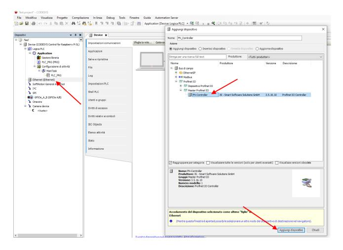
Double click on Ethernet, set the Ethernet port and the IP address of the PLC (in this case use 192.168.90.44):
