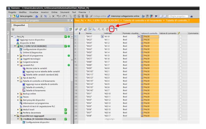
Under the "Control value" column you can read the I/O value in real time.
