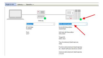
Now that the PLC has been detected, move on to insert a Profinet port on standard Ethernet: Right click on device and "add device":
