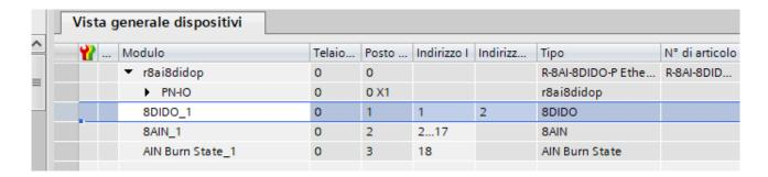
So byte I1 contains the 8 digital inputs (those as inputs), byte Q2 the 8 outputs (those configured as outputs). Bytes from I2 to I17 show the values of the 8 analogue inputs (2 bytes per input). Byte I3 shows the burnout status of the analogue inputs.
