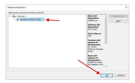
The PLC is now connected to the system:
