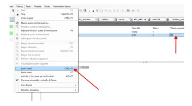
And then with "Write values" all the outputs are activated correctly.
