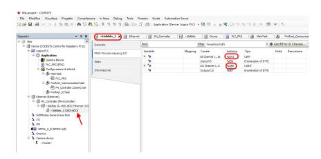
Declare an 8-bit (Word) variable for the 16 inputs and one byte for the 8 outputs. In the program, instead, read the inputs from %IW2 and write the outputs on %QB0:
