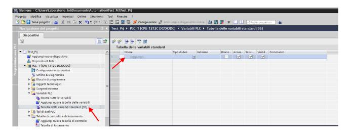
Add the tags related to the IO (in the example it is an R-16DI-8DO that is 16 digital inputs and 8 digital outputs). The addresses are written here:
