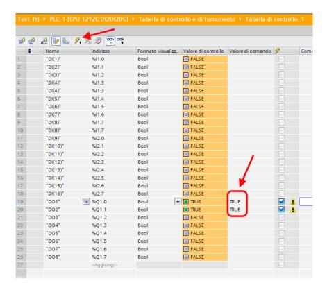
In the "Control value" column, the outputs are now correctly read to "True".
