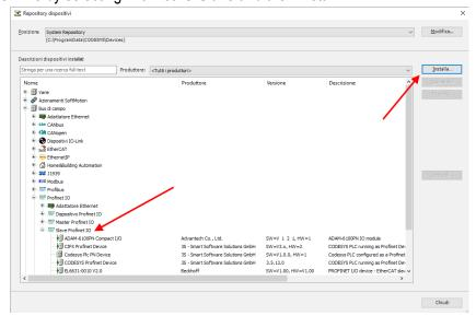
Now point to the correct folder and press OK. Codesys has now added the GSD file correctly.
