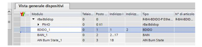
So byte I1 contains the 8 digital inputs (those as inputs), byte Q2 the 8 outputs (those configured as outputs). Bytes from I2 to I17 show the values of the 8 analog inputs (2 bytes per input).
