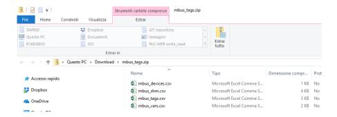
Two of these files are to be used in Straton: mbus\_shm.csv (the shared memory configuration) mbus\_vars.csv (the M-Bus vars) At this point, perform the following steps:
