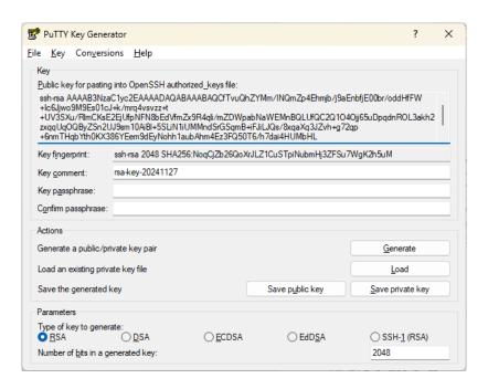
The public key appears in the textbox, which must be copied to the device; do not save the key by pressing the button but copy/paste it into a new file, making sure to select the ENTIRE key:
