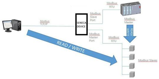
In this case, one serial port is configured as Modbus Slave and another is configured as Modbus Master.
