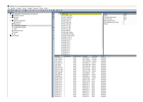
If we want to create a tag that can be written by Straton and displayed for example on the physical or virtual display, we must first create a TAG of the "internal" type in "shared memory" and enable the export to Display/PLC:
