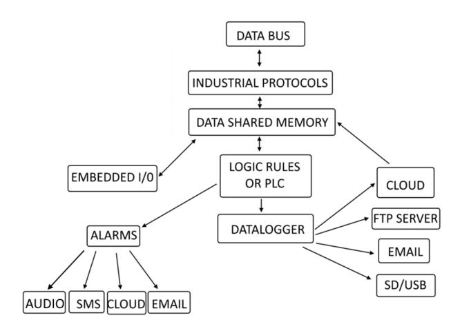
The acquisition of data (Tags) in the buses (Data Bus) takes place via industrial protocols (Industrial Protocol) or via direct acquisition of the integrated I/Os (Embedded I/O).
