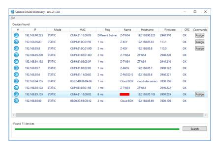
This application shows the IP address, MAC address, FW version and some other useful information, for each SENECA device connected to PC.
