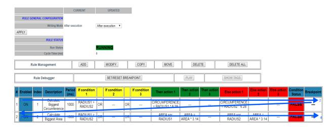
When all the rules are executed, the execution starts again from the first one. More in detail the correct diagram is:
