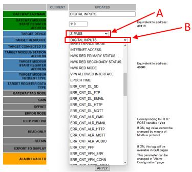
In addition to the embedded IOs, tags are available for GPS position, redundancy, VPN and error counters.
