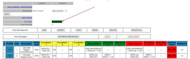
To test the program we can write the tags RADIUS1 and RADIUS2 from Modbus RTU / MODBUS TCP-IP (registers 40100-40101 in our example) or using the "Tag View" page:
