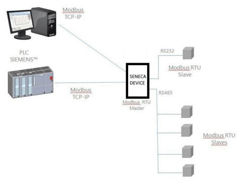
In the figure above, two serial ports are configured as Modbus RTU Master.
