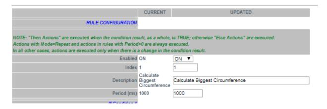
Then we add the "if condition" to determine which is the larger radius between the two provided (we only need 1 if condition):
