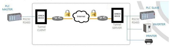
The point-to-point serial tunnel allows to extend a serial connection between two serial devices (that support the same protocol) via a TCP/UDP connection.
