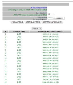
The baud rate value shown in the table header reminds you of the parameter choice for the last scan procedure. The table with the detected M-Bus devices is stored permanently, so after switching the device off and on again the results of the last scan are still available; they will be overwritten by the next scan or deleted by a factory reset.
