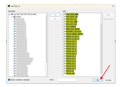
At this point the TAGs are imported into the PLC, note how all are set by default as ReadOnly:
