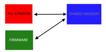
In this mode it is possible to activate the data logger, alarms, display / virtual display and communication protocols already present in the firmware and to read and write the TAGs directly from the PLC.
