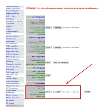
Press the "LOAD" button to load the selected file. The following screen appears:
