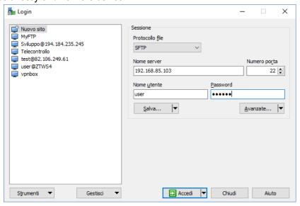
The WinSCP program is used to transfer files from/to the device.
