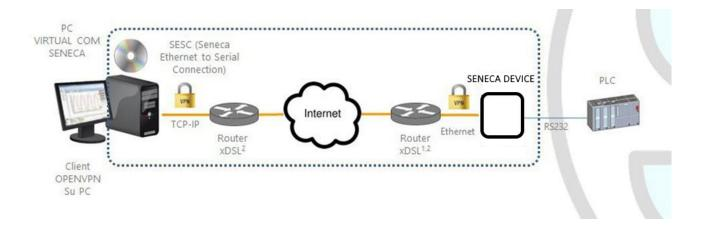
The Virtual COM with RFC 2217 support feature allows a PC application, which transmits data only on a serial line, to communicate with a remote serial device, using Ethernet/Internet; in other words, through the Seneca device, a PC and a serial device, located in distant sites, can communicate because they are directly connected.
