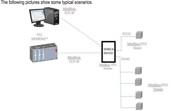
In the figure above, two serial ports are configured as Modbus RTU Master.
