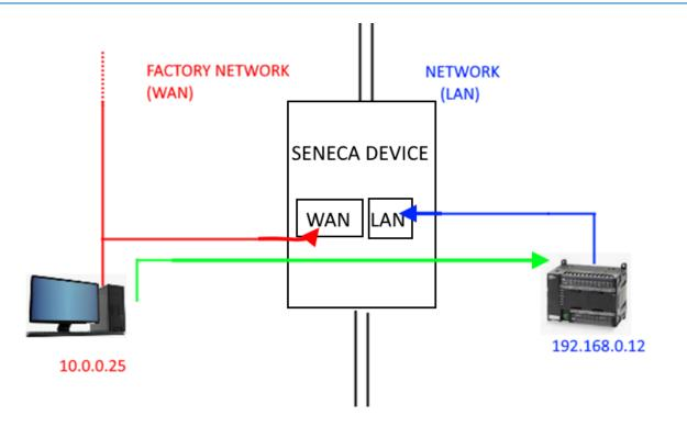
It is necessary to create a new address (10.0.0.26) which is located on a PC-compatible network (10.0.0.25).
