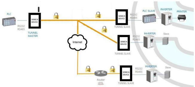
The Serial Tunnel Point-to-Multipoint allows you to create a tunnel with a master and more than one slave; on the master side, the data received from the serial line are sent to all the slaves, via the *multicast* transmission mode, in UDP packets.
