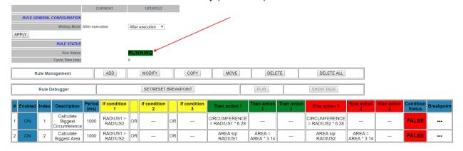
To test the program we can write the tags RADIUS1 and RADIUS2 from Modbus RTU / MODBUS TCP-IP (registers 40100-40101 in our example) or using the "Tag View" page:
