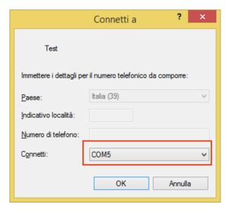
COM5 is now connected to the Seneca device by a TCP connection to port 8000.
