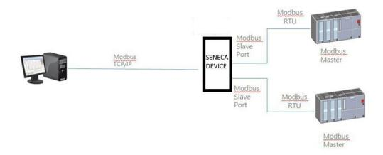
In the figure above, two serial ports are configured as Modbus Slave and connected to a Modbus Master PLC port; in this way, the two PLCs and the Modbus TCP Client can write/read the shared memory to share data.
