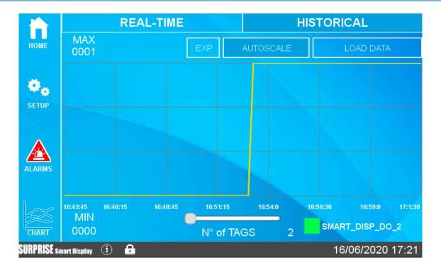
In case a USB disk is connected, it is possible to export to a file the chart values displayed, by pressing the "EXP" button.
