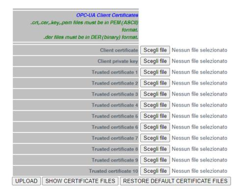
The "Choose File" button selects the certificate. These are only uploaded to the device after pressing the "Upload" button.
