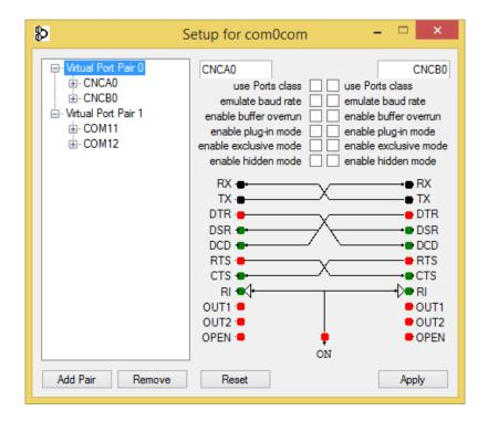
During installation two pairs of virtual COM are created: CNCA0, CNCB0 and also:
