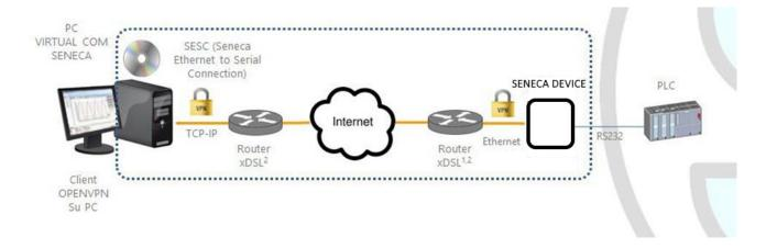
The Virtual COM functionality allows a PC application, which transmits data only on a serial line, to communicate with a remote serial device, using Ethernet/Internet; in other words, through the Seneca device, a PC and a serial device, located in distant sites, can communicate as they are directly connected.
