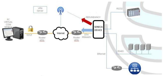
"Network redundancy" is a feature that can be enabled on devices where a mobile or WI-FI modem is available.
