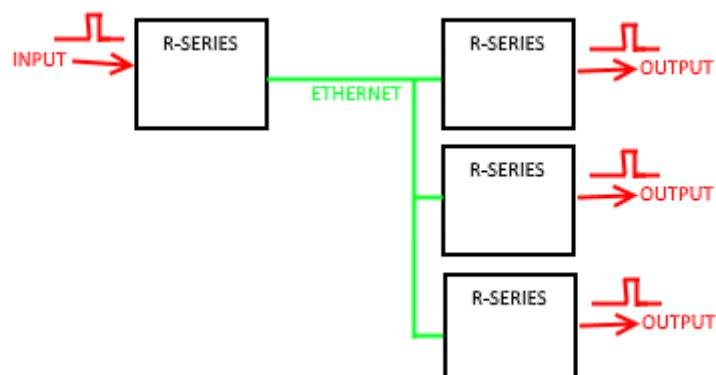
Each R-series device can send and receive a maximum of 32 inputs.
