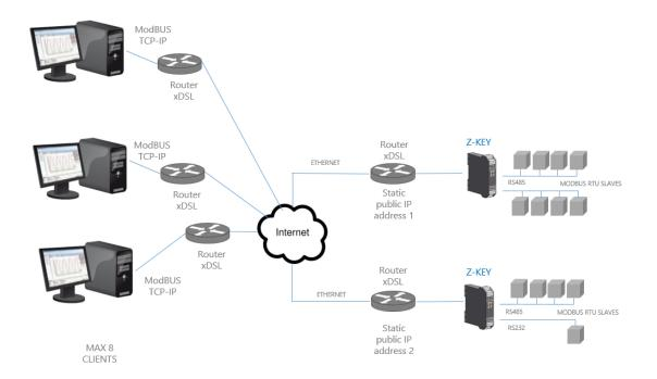
A maximum of 8 simultaneous Modbus TCP-IP Clients are supported.
