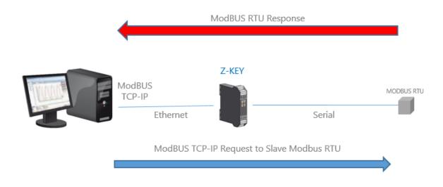
The Modbus TCP Client requests the reading/writing of a Modbus register via Ethernet, the gateway converts the request towards the serial slaves in Modbus RTU/ASCII and the Modbus RTU/ASCII response of the interrogated slave is subsequently converted towards the Modbus TCP Client.
