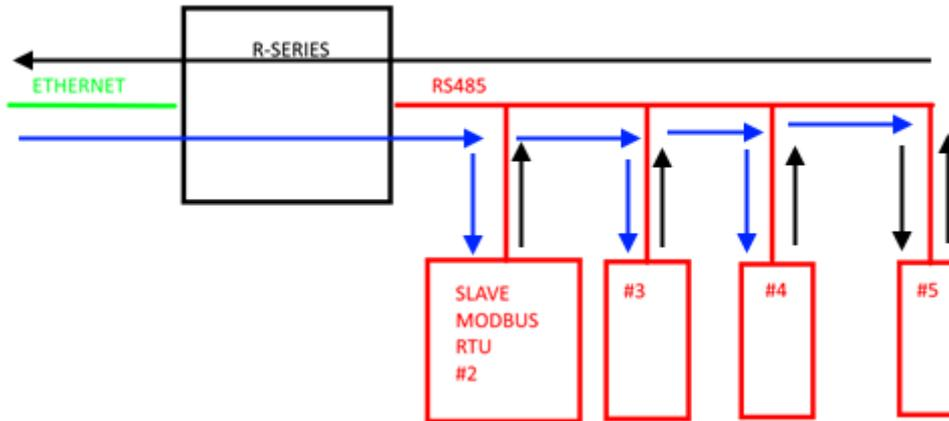
Each Modbus TCP-IP request with station address other than that of the R series device is converted into a serial packet on the RS485 and, in the case of a reply, it is turned over to TCP-IP. Therefore, it is no longer necessary to purchase gateways to extend the I/O number or to connect already available Modbus RTU I/O.
