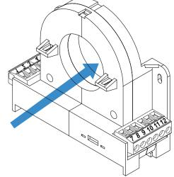
instrument, creating a series of loops. The current measurement sensitivity is proportional to the number of cable passages through the hole.
