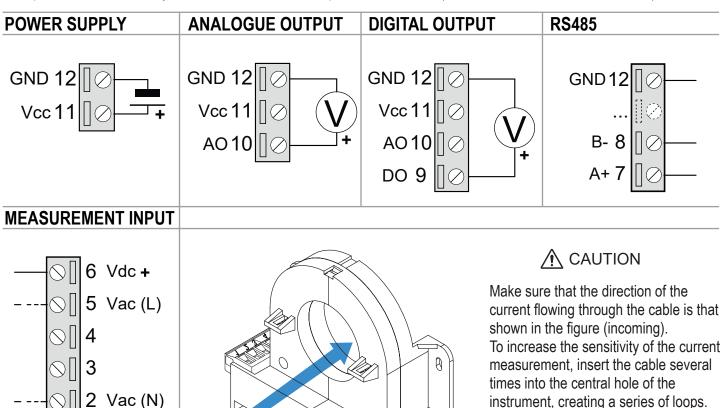
Connect just a pair of terminals for the measurement.
