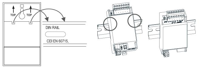
**Installation:** Position the device on the OMEGA rail resting the upper teeth from top to bottom. Push the lower part towards the rail until the locking system engages.
