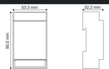
Dimensions: 53,3 x 90 x 32,2mm, Weight: 80 g; Case: Self-extinguishing UL94-V0 PC / ABS material SIGNALS VIA LED ON FRONT PANEL
