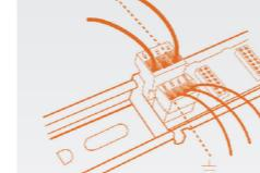
Power supply and data transmission are ensured by modular bus support (RS485) from DIN rail in 1, 2, 4, 8 slots. Alternatively, depending on the models, power supply and data transmission are distributed via terminals or IDC10 connector.
