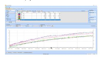
Trend Viewer is the software that complements Data Recorder and allows you to consult the databases with the recorded data and display them in charts that can be customized in colours, filtering the data by channel and by time intervals.
