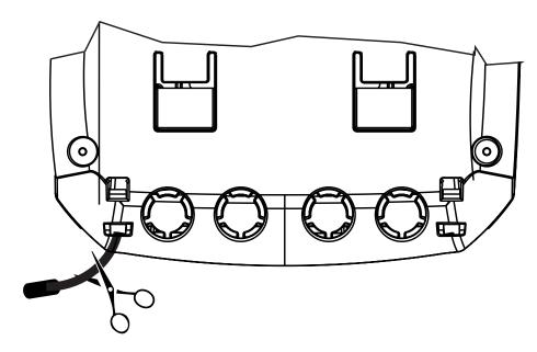
Once the pre-installed probe has been removed, connect the NTC-150 probe by wiring the cables to the Moretti 12 and 13 as shown in the figure below.
