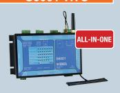
Modular automation solution able of managing 100 tags for universal applications. Strong of high connectivity thanks to FTP client. SMTP client, http, ModBUS TCP, ModBUS RTU protocols, the controller also has on board 2 analog inputs at 16 bits configurable in voltage or current and can realize automation systems expandable with ModBUS I/O modules / thernet Z-PC Line.
