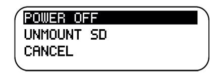
To choose the desired command use the SCR key which allows you to scroll through the various options, to confirm the desired option press the PWR key.
