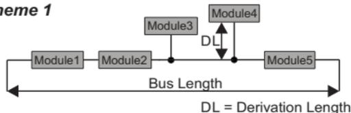
For the best performances, the use of special shielded cables is recommended (BELDEN 9841 cable for example)
