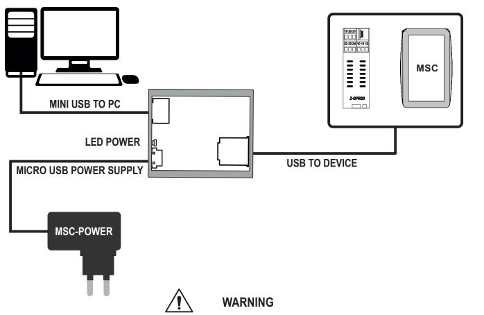
If you need to use USB-ISO isolator with the MSC calibrator please use the power supply (MSC-POWER) supplied with the MSC calibrator in order to avoid reading errors or malfunction of the instrument.
