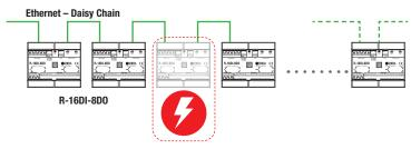
Ethernet connection and data transmission are active even in case of failure or power failure of a module in the chain. In this way the availability and continuity of the service are quaranteed.
