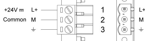
DC Power Connector - AWG24 wire size - R/C Terminal Blocks (XCFR2), Female pitch 5.08mm, torque 4.5 lb-in (50Ncm)
