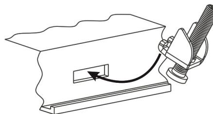
Tightening torque: 75 Ncm
