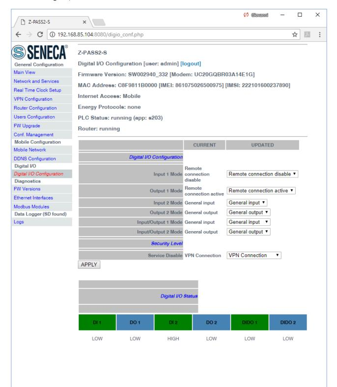
The status of the digital input configured as "Local Alarm" is reported in the "ALARM" column in the "Devices" tab of the "Seneca VPN Box Manager" and "Seneca VPN Client Communicator" applications.
