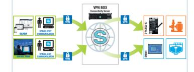
In Telecontrol / Single LAN mode (Always ON connection) VPN BOX works like a network server which is assigned a static public IP. Communication is simultaneous and always active between all remote sites and the server, as well with the different subnets that are part of the overall system.
