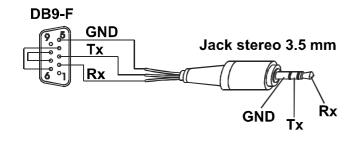
The connection cable DB9 with a 3.5 mm stereophonic jack, can be assembled as indicated in the following figure, or can be bought as an accessory (see *Accessories*).
