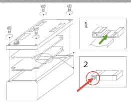
After removing the 4 screws with a screwdriver, follow the instructions in the picture above: to insert the SIM card, follow figure 1; to remove it, press the button on the side of the slot as shown in figure 2.
