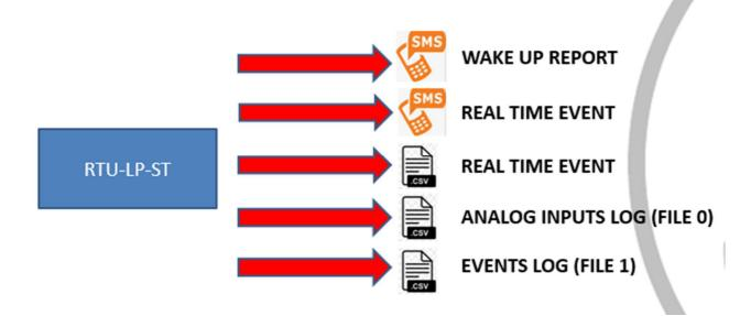
RTU-LP-ST device can receive the following type of data:
