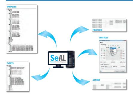
SEAL (SENECA Advanced Language) is a software designed for advanced management of automation and remote communication projects. SEAL allows you to intuitively manage variables, commands, automations, alarms, thresholds, reporting, network of communication with the possibility of configuration and remote update via SIM or Ethernet.
